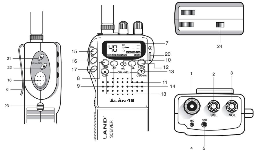
1. **Antenna connector:** insert in this plug the antenna supplied with the radio. It is possible to use external vehicular antennas to obtain a better performance.
